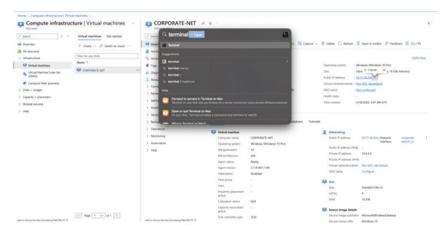
29) Once the terminal has opened, type "ping" press spacebar and then enter the public IP address for the virtual machine. Click enter and you should see bytes being returned from the IP address.
