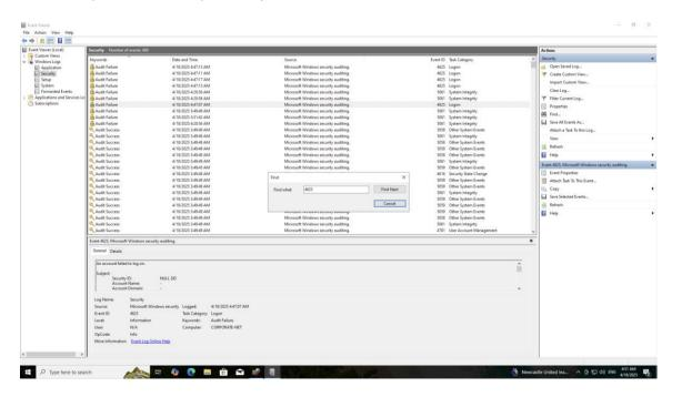
The logs can be filtered using the filter current log tool to the right of the screen.
